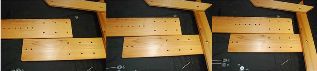
Now that you have chosen a roof height, layered the upper leg on top of the lower leg while aligning their bolt holes, complete the leg section by installing the following 5 bolts: Foot to diagonals, diagonals to upper and lower legs and the lower leg to foot. Install washers and wingnuts but leave slightly loose. Complete the other leg assembly and you will be ready to add the trough.
