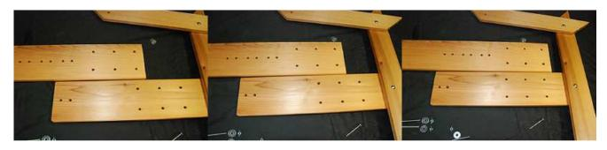
Now that you have chosen a roof height, layered the upper leg on top of the lower leg while aligning their bolt holes, complete the leg section by installing the following 5 bolts: Foot to diagonals, diagonals to upper and lower legs and the lower leg to foot. Install washers and wingnuts but leave slightly loose. Complete the other leg assembly and you will be ready to add the trough.
